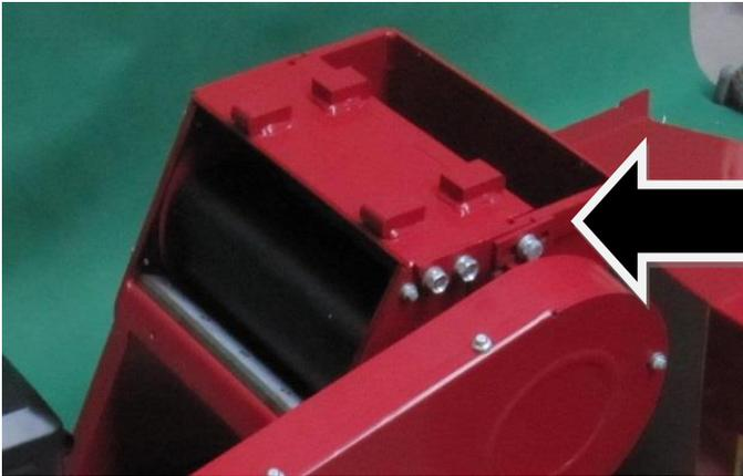
Lugs on body of the machine for Feed & Discharge chutes.
