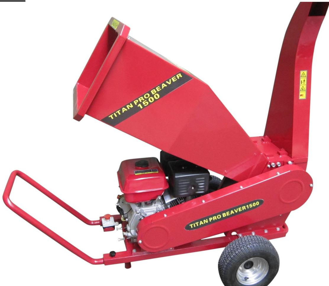
11. Fill with horticultural engine oil using a small funnel up to the threads in the filler hole. Use sae 30
