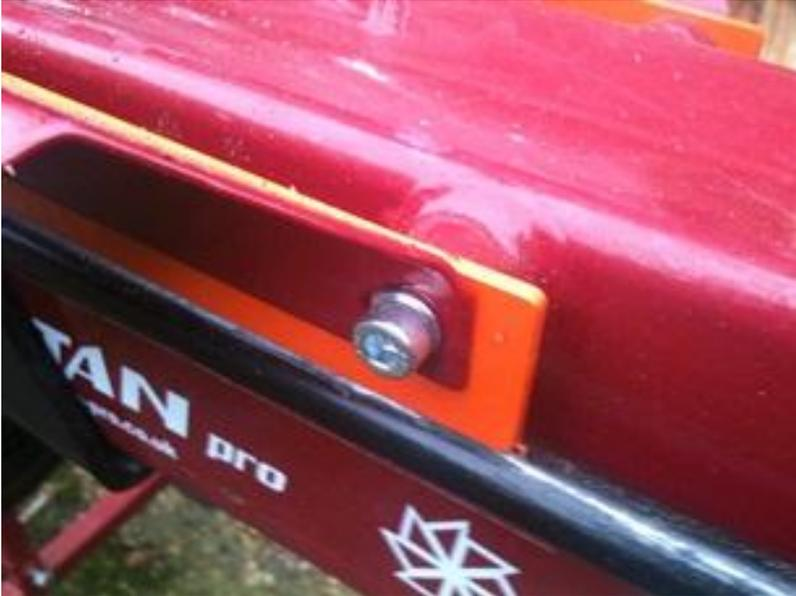
4. Install horizontal rails between the side wing and the body of the machine. Use all **new** bolts and washers supplied
