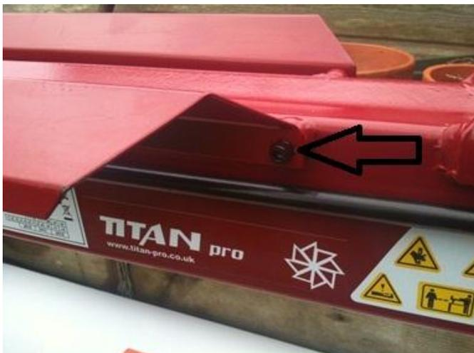
3. Remove the back bolt from side wing and center bolt.(you will use new bolts and washers supplied)
