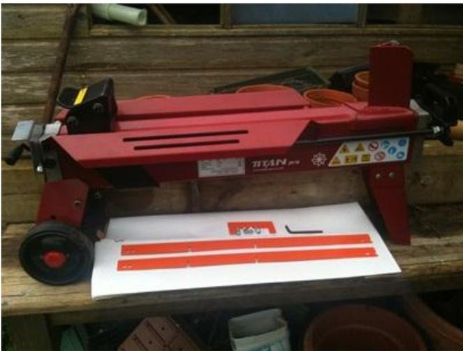
2. Start with one side first, remove the front bolt of the side wing as shown in photo below and discard bolt (you will use new bolts and washers supplied)
