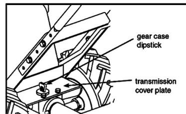
you add to the front transmission, you must wait a short period of time for the oil to follow rearward and equalize in both front and rear. The dipstick will read correctly on level ground for both gear units.
