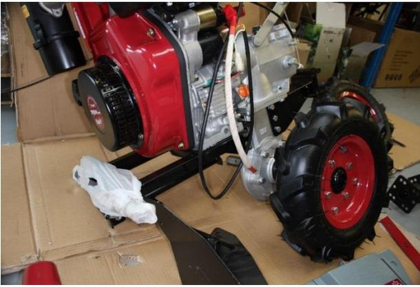
3. Lean Machine to the left and slide on right hand wheel
