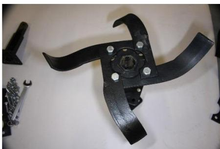
Repeat this to place all four tines around the bar. Bolt all four corners tightly.
