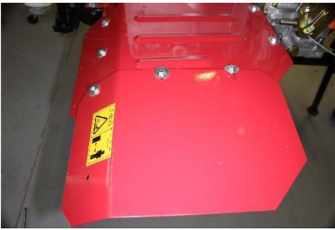
16. Slide right hand outer tine cover under 3 bolts and tighten to secure in place. Repeat on left side.
