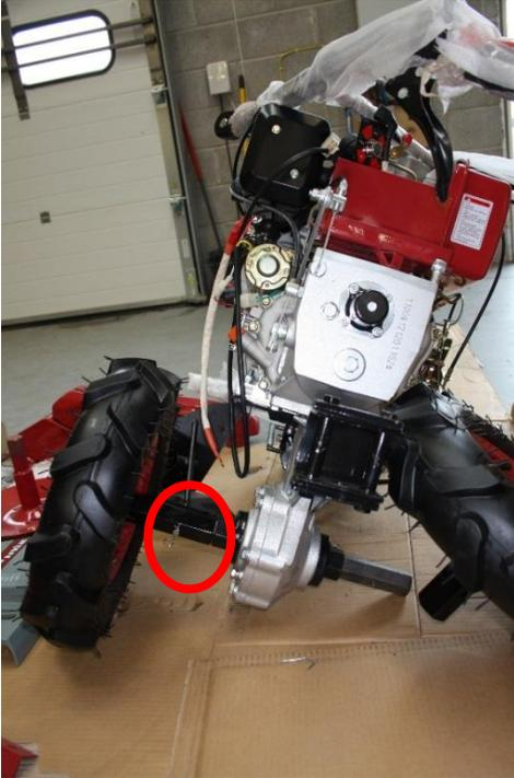
4. Insert Pin (shown below) into shaft as shown to secure wheel (Left)
