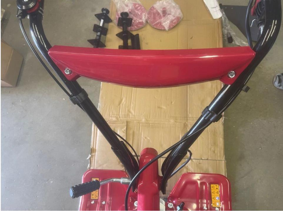
Next, fit the belt cover. This should line up with the static parts of the machine and can be secured with the three-pronged bolt shown in the centre of the picture below.
