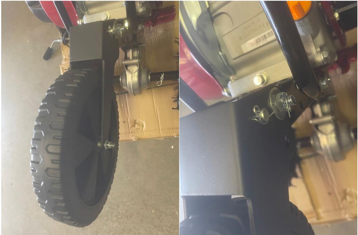
After affixing the front wheel, the machine will now be stable to sit on the three wheels.
