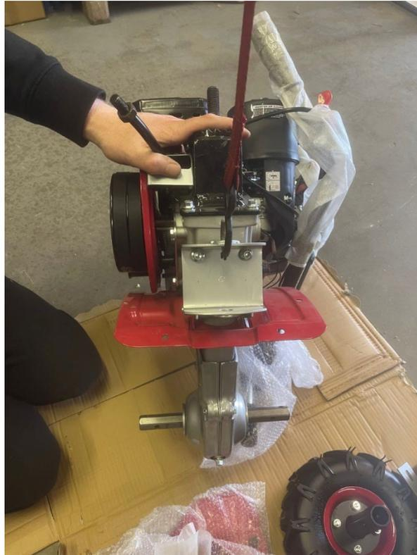
After sliding a wheel on, secure this using the pin and r-clip mentioned previously. When both are in place, it will appear as below. It is also important to ensure the tread on your wheels faces the correct way (again, as shown below.)
