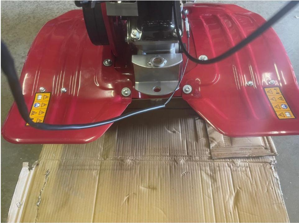
This bracket sits underneath the mudguards. As seen in the image above, there are four bolts, two on either mudguard which the bracket is secured by. The image below shows the bracket secured in place.
