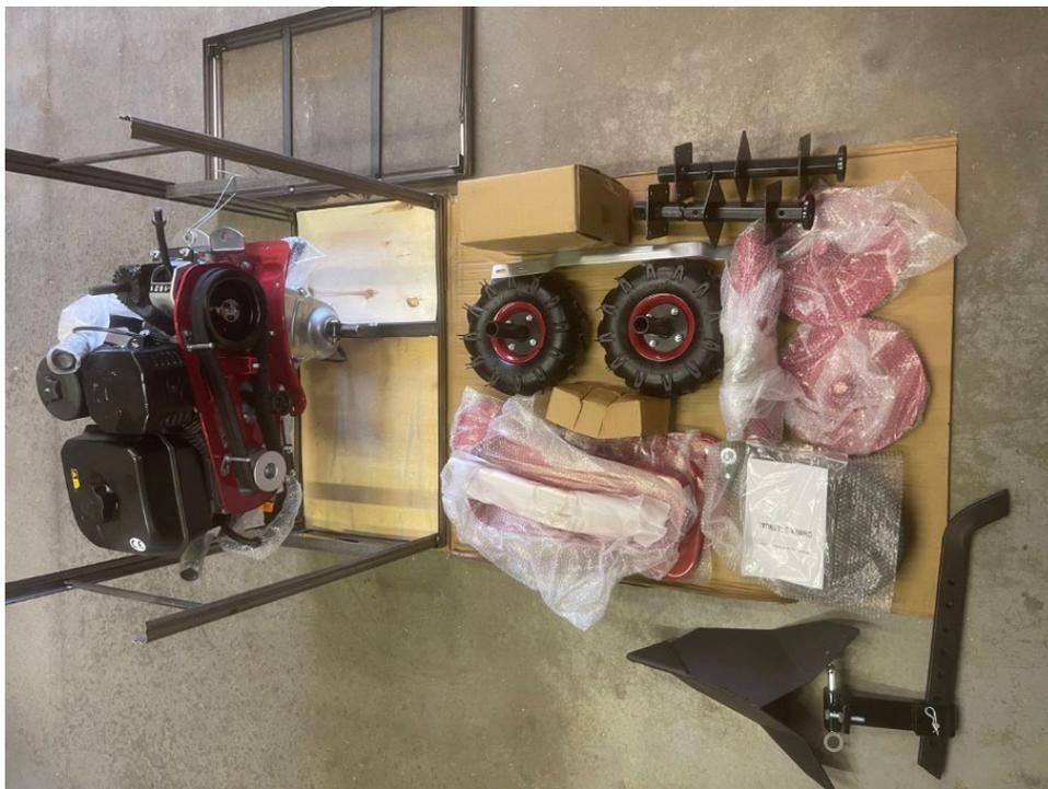
First, remove the outer cardboard packaging to gain access to the metal cage and contents. This image also shows the ridger attachment – this item is sold separately but included here for completion. You can also remove the top of the metal cage to increase your access at this point.
