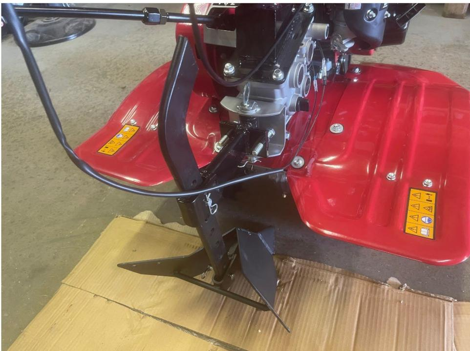
The final step of the main body build is attaching the gear lever. The handle extension screws on to the bottom part of the lever which is already in place at the gearbox shifter.
