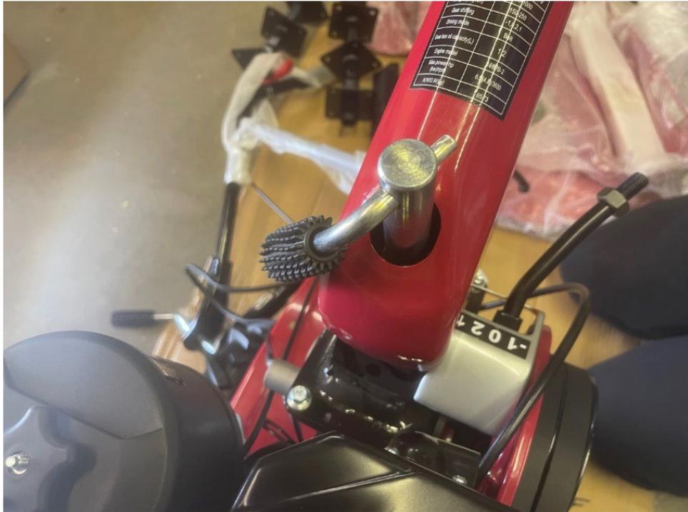
The next step is to attach the handlebars (upper and lower parts). These are secured by tightening the handle lever at the bottom where it seats onto the chassis, as pictured above. You can then secure the handlebars at the top to the bottom section, as shown below.
