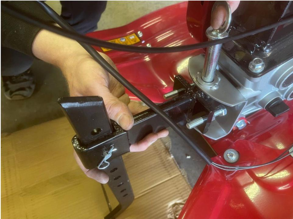
This rod can also be turned upside down, with the curved end at the uppermost point to utilise this with the ridger attachment (sold separately.)
