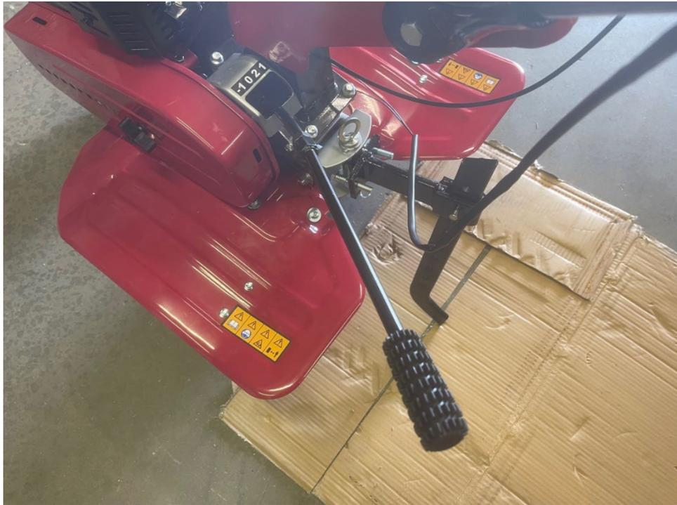
Now that the build is complete, you can add the engine oil and gearbox oil to the machine. Firstly, the engine oil can be added to the fill plug area as shown in the picture below. We recommend SAE30 engine oil; you will require approximately 0.6 to 0.65 litres of oil. A sticker showing how and where to fill the oil to is also displayed on the belt guard cover, next to the fill plug.
