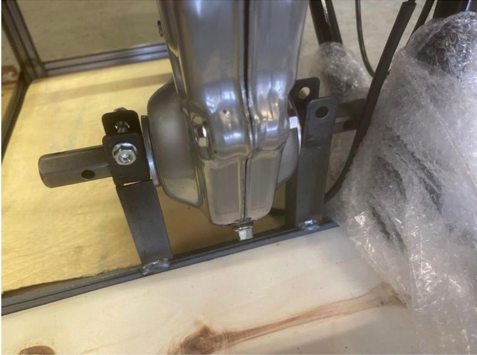
Next comes removing the chassis and engine of the machine from the cage. This will require two people to lift this out. As pictured above, the axle is bolted into two brackets to ensure the machine doesn't move in transport (one of these have been removed in the image to illustrate.) To undo these bolts, you will require a 13mm spanner, which can be found in the toolkit. After undoing these bolts, you can now lift the machine.
