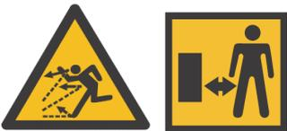
Danger or injury from flying parts! Never point the discharge chute towards bystanders. Always maintain a sufficiently safe distance. Be careful to prevent debris, such as stones or twigs being thrown from the mower.
