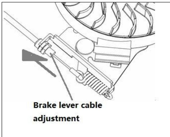
Engine brake adjustment:
