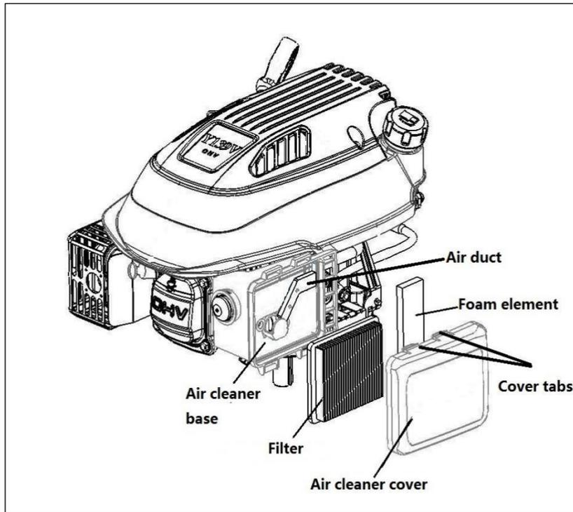
Where paper filters are fitted, excess dust and dirt may be removed by tapping it on a hard surface several times or blowing compressed air onto the filter.
